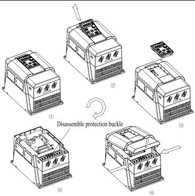
Fig. 2-7 Disassembly schematic diagram of 5.5kW-7.5kW
