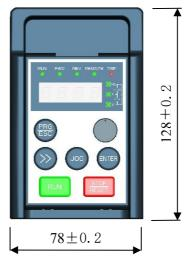
Fig. A4-2 Keypad's tray Installation Dimension (Unit: mm)
