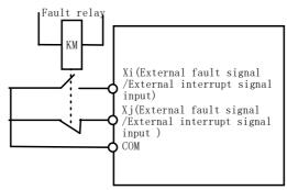
Fig. 5-3-6 Normally open / normally closed
