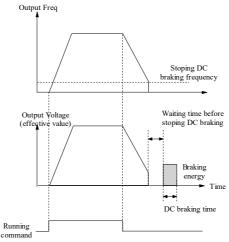
Fig. 5-1-7 DC braking
