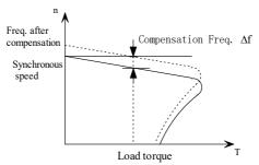
Fig. 5-9-4 Auto slip compensation diagram
