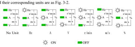
Fig. 3-2 Combinations of unit indicator and their means
