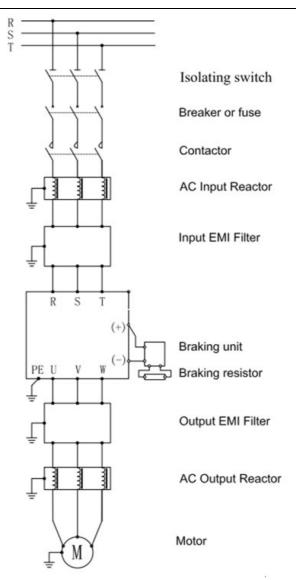
Fig. 7-2 3018G/3022P and above Peripheral Equipment Connection Diagram
