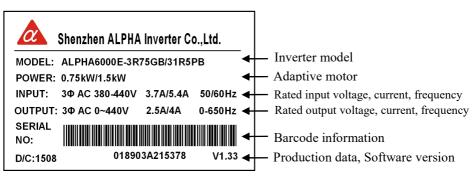
Fig. 1-2 Nameplate of Inverter
