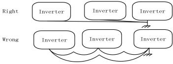
Fig. 2-14 Earthing Connection Method
