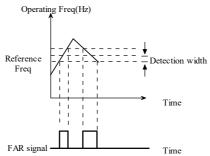
Fig. 5-3-8 FAR detection diagram
