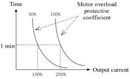
Fig. 5-13-1 Motor overload protection curve
