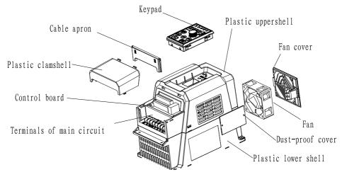
Fig. 2-3 Main parts of 4kW and below
