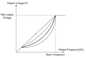
Fig. 5-9-1 Torque-reducing curve
