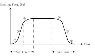
Fig. 5-1-6 S-curve acceleration/deceleration
