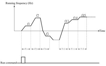
Fig. 5-5-2 Holding the frequency after single cycle
