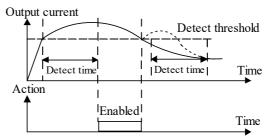
Fig. 5-13-2 Overload pre-alarm function
