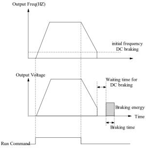
Fig. 5-3-5 DC braking
