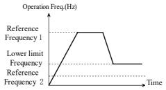
Fig. 5-2-3 Running at lower limit frequency
