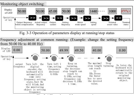
Fig. 3-4 Flow chart of frequency setting
