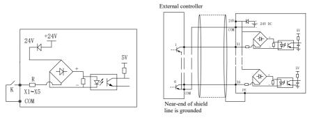
Fig. 2-21 Wiring diagram of multi-function input terminals
