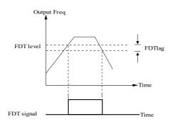
Fig. 5-3-9 Frequency detection FDT
