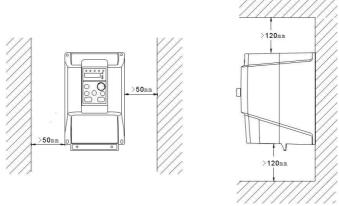
Fig. 2-2 Installation Direction and Space
