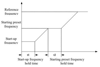
Fig. 5-1-4 Starting preset frequency and hold time
