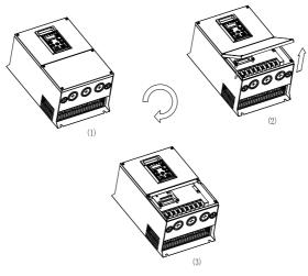
Fig. 2-8 Disassembly schematic diagram of 11kW-160kW
