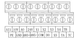
Fig. 2-15 Terminal arrangement of S2R4GB~S2R75GB
