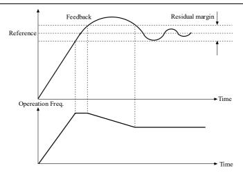
Fig. 5-7-1 Residual margin diagram
