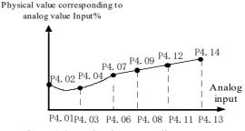
Fig. 5-4-2 Analog input non-linear curve
