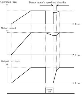
Fig. 5-1-2 Rotating speed tracking restart
