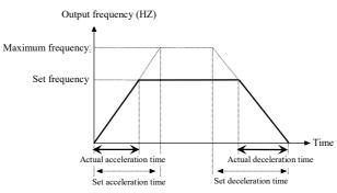
Fig. 5-1-5 Linear acceleration/deceleration
