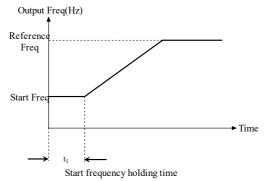
Fig. 5-1-3 Starting frequency and starting time
