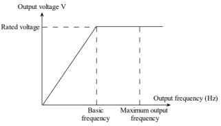
Fig. 5-0-1 Relationship between output frequency and output voltage
