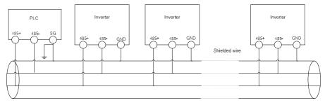
Fig. 2-20 Recommended wiring diagrams (inverters and motors are all well grounded) when PLC is in communication with multiple inverters
