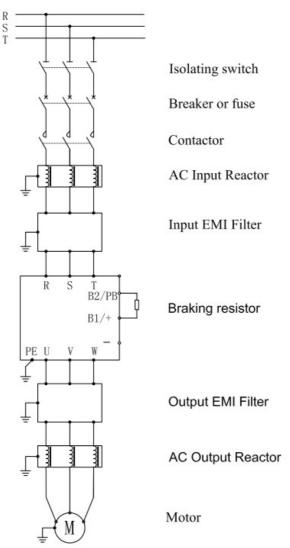
Fig. 7-1 S2R4GB~3015GB/3018PB Peripheral Equipment Connection Diagram
