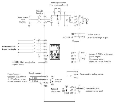
Fig. 2-24 wiring diagram
