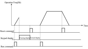
Fig. 5-3-1 Terminal reset
